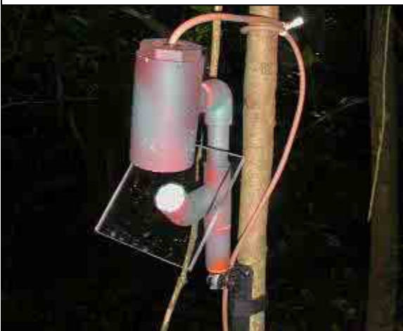
Figure 15. Receiver section of an acoustic trap
