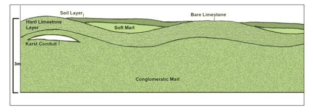
**Figure 9:** Schematic Geological Cross Section of Bedrock of the area (Information compiled from several quarries and test pits in and around the area; Holland, pers. com.)
