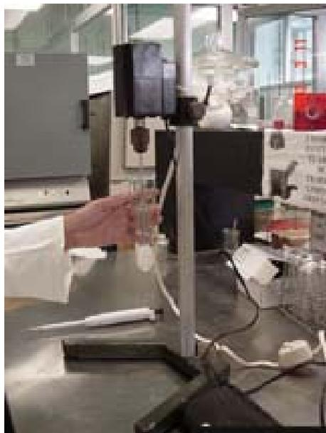
**Figure 6.1** Tissue homogenizer built with a sewing machine motor (Photograph courtesy of Gabriela Rodríguez-Fuentes)
